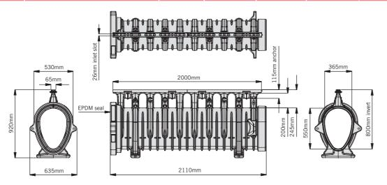
ACO Qmax® 550 with ACO Q-Flow ductile iron edge rail
