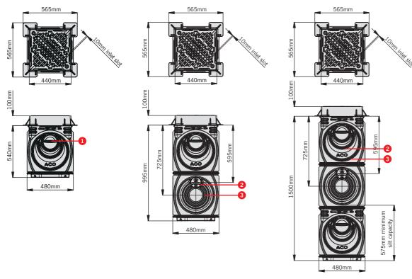
Image shows ACO Qmax® 225 and 350 access chamber Load Class F 900.
