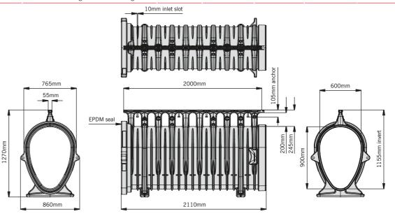
ACO Qmax® 900 with ACO Q-Guard galvanised steel edge rail
