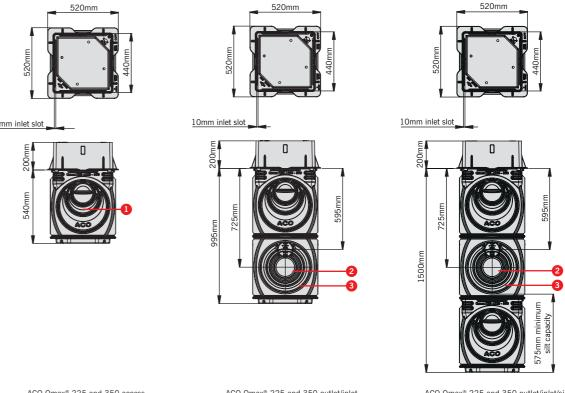
ACO Qmax® 225 and 350 access chamber with D 400 ACO Q-Slot
