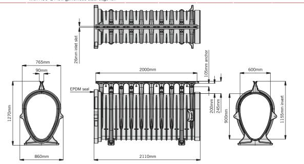
ACO Qmax® 900 with ACO Q-Flow galvanised steel edge rail
