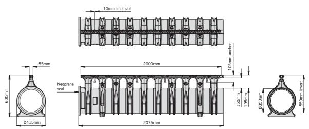
ACO Qmax® 350 with ACO Q-Guard galvanised steel edge rail
