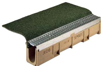
The units feature an integral metal edge cast into the channel. This edge is used to fix the carpet, and is independent of the grating. This means that when the grating is lifted for cleaning or maintenance of the channel, the carpet will remain fixed in place.
