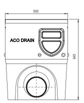
Size of the sump unit ACO Drain® Monoblock PD 200V
