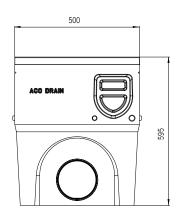
Size of the sump unit ACO Drain® Monoblock PD 150V
