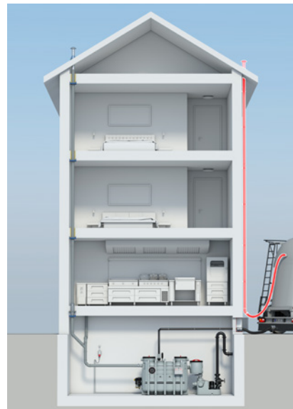
Separate pendulum gas pipe above the roof
