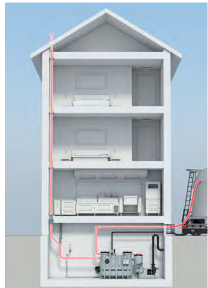
Pendulum gas line connected to grease separator
